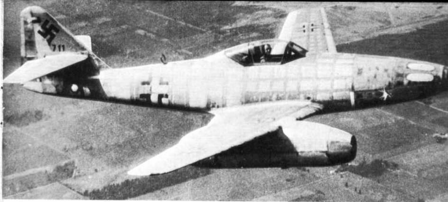
Me 262A-2a, Werk. Nr. III711, shows clearly its broad triangular fuselage and sharply swept wings. Lower: An Me 262 caught by the camera gun of a P-47 Thunderbolt.
