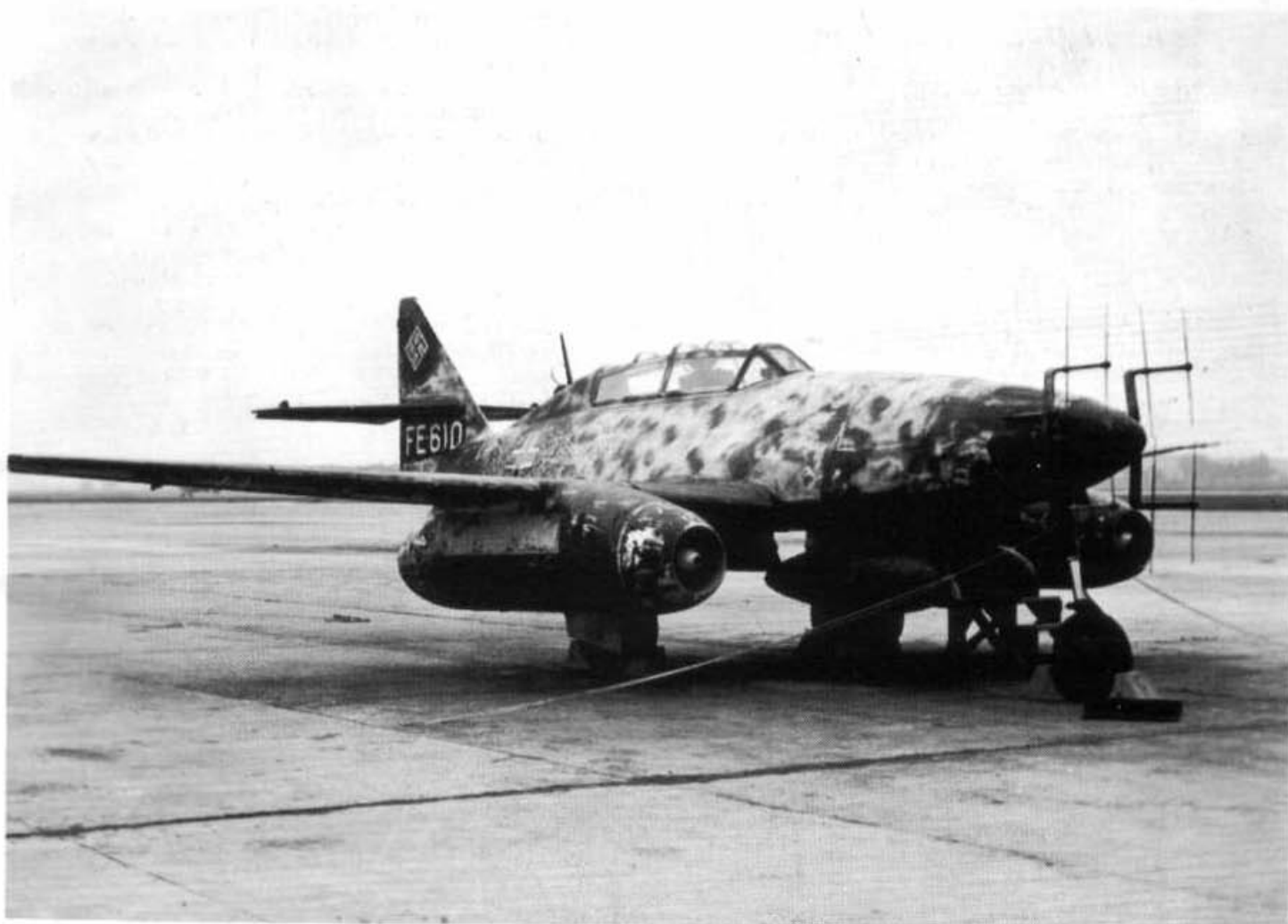
The blanked off upper cannon ports and the long barrellled 20 mm. MG 151/20 cannon are shown here.
