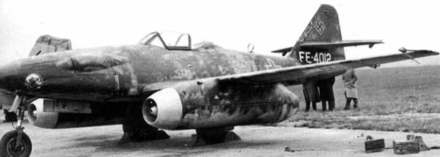
Me 262A-1a/U3 showing clearly its large blister fairings for the RB 50/30 cameras.
