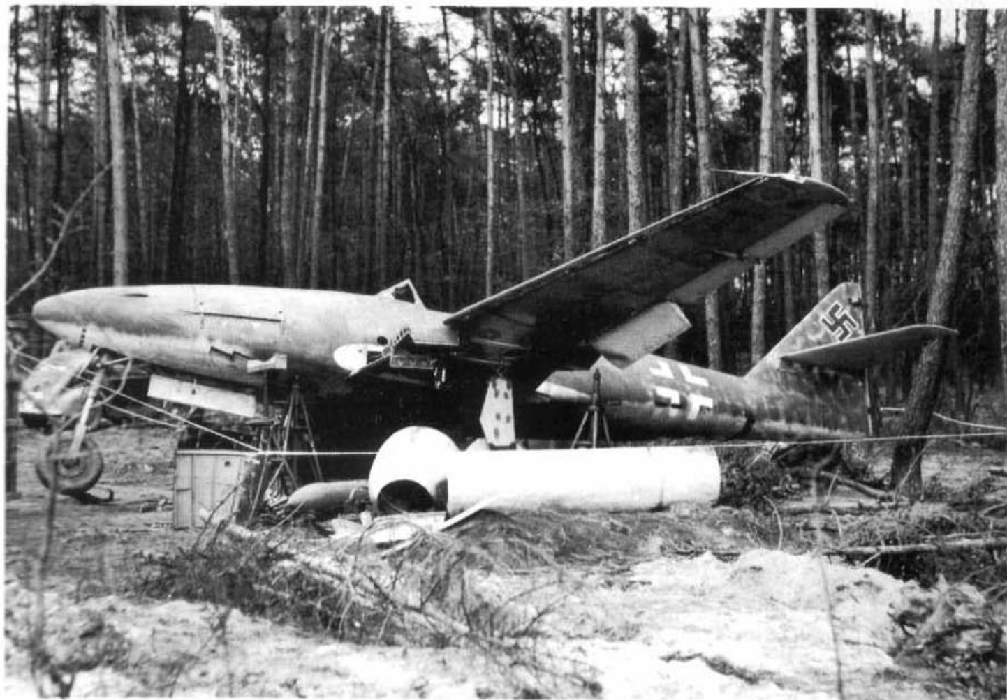
An Me 262A-1a in a state of disrepair. The dotted trestle marking on the underside of the nose is standard but the one under the rear fuselage is unusual. The national marking on the fuselage is lower than usual. Note the lack of any underwing marking.
