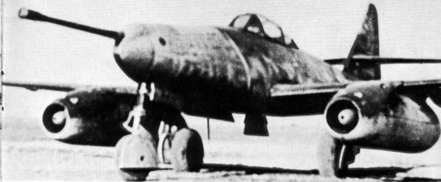
The original prototype MK 114 installation showing the blister type fairing which obscured the camera gun window in the nose cone.
