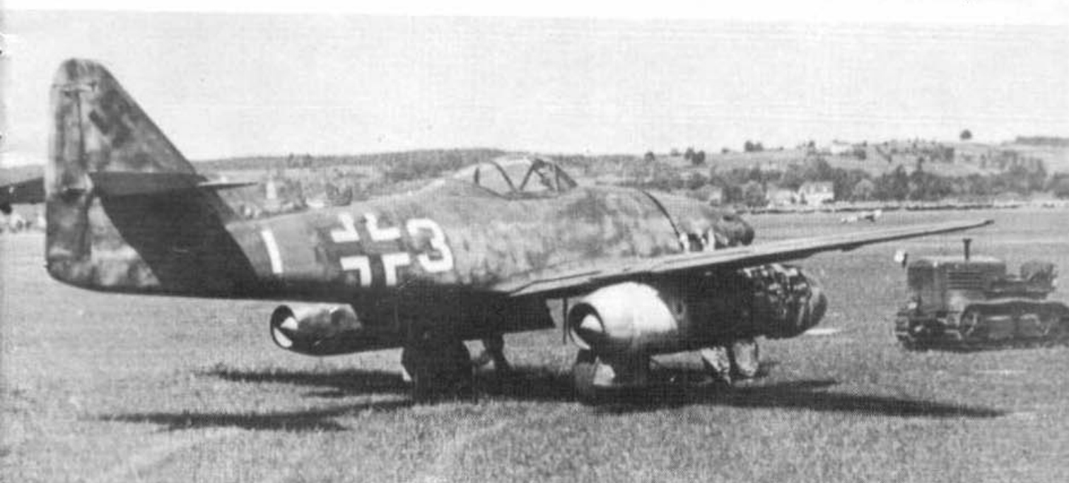
The slight inaccuracy of the fuselage cross shown here is due to misalignment of the fuselage access panel.
